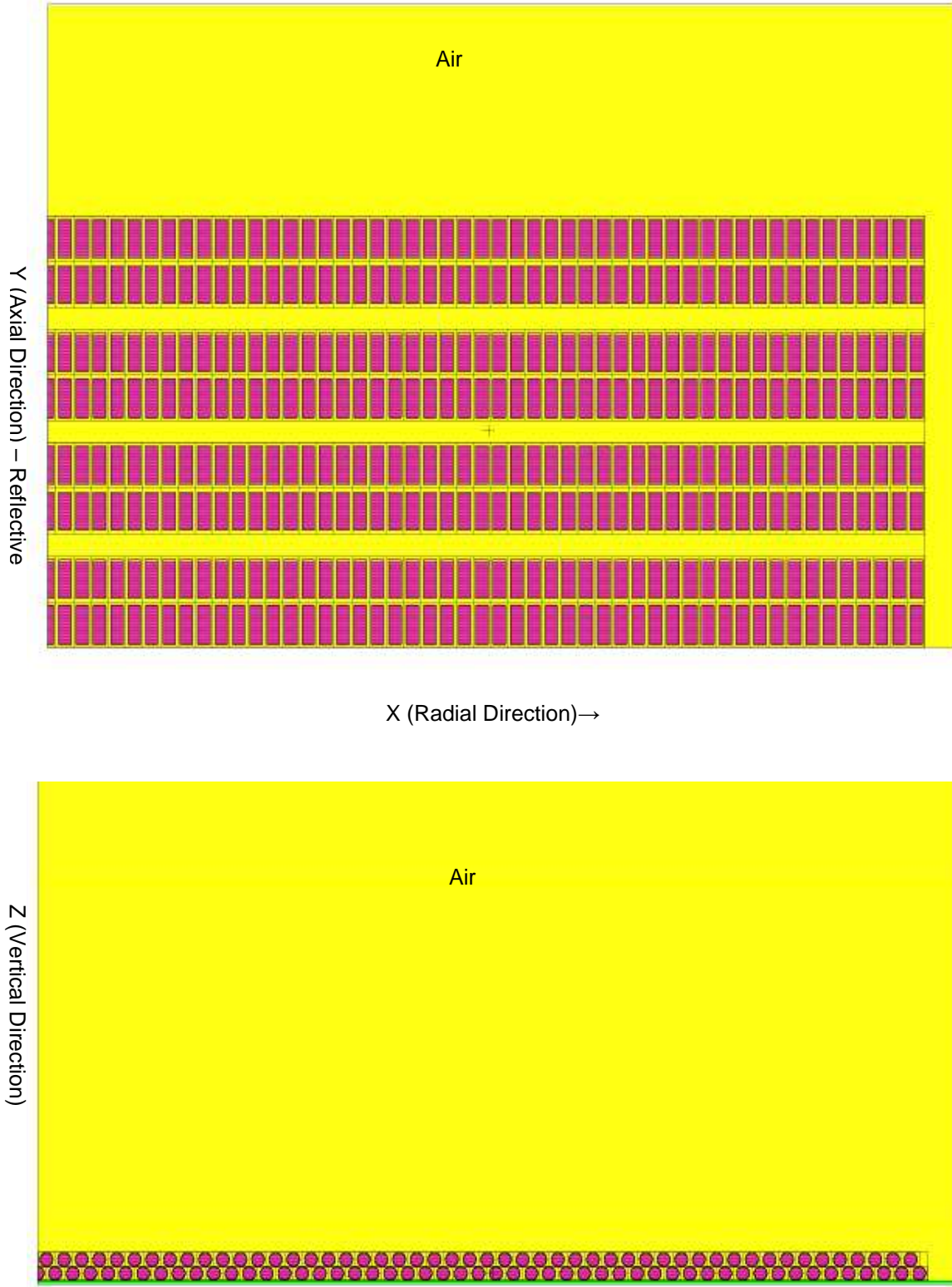
Figure 8-1 UUSA UBC Storage Pad Validation Model
